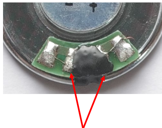
DON'T solder to these pins
